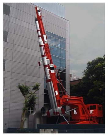
The Lambda 4S or L-4S was an experimental Japanese expendable carrier rocket. It was produced by Nissan and the Institute of Space and Astronautical Science and launched five times between 1966 and 1970 with Osumi technology demonstration satellites. The first four launches failed, however the fifth (L-4S-5), launched on 11 February 1970, successfully placed Ohsumi (Osumi-5), the first Japanese satellite, into orbit.
